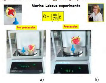
Fig. 1. a) 3-D Gyro at rest with an initial weight of 46.45 g; b) 3-D Gyro in precession weights at 46.3 g.
